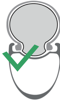
The tube is completely between the tire and rim.
